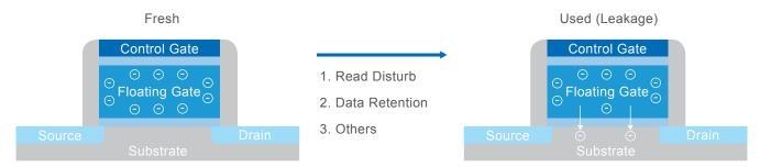
Potential Failure Mechanisms
